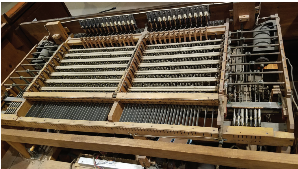
1. A look at the current mechanical combination action. An early “computer”.
